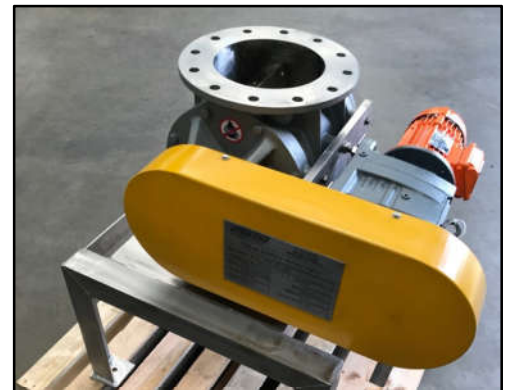
Stainless Steel rotary valve to ensure consistent flow of product from separation bin and to control airflow into silo downstream.
