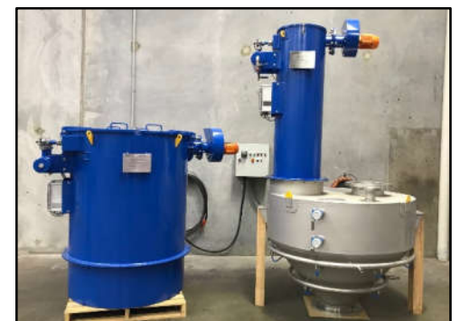
Pictured above, dust extractor and buffer hopper to surge fill vessel for conveying efficiency.
