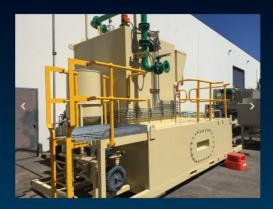
Different flocculants have varied properties which meant the design of the flocculant production plant must consider the addition and mixing specific to the applied product and the water treatment required. Lime System's build small skid mounted packages through to large scale fixed plants. Lime Systems plant has been used for clarifiers, thickeners, waste water treatment and drinking water treatment among many other process modification and treatment requirements.
