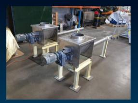
All screws are of heavy duty, mining industry construction with specialised shaft sealing, grease purged labyrinths and outboard mounted ball bearings. Lime Systems — Bulk Storage Solutions incorporate best in class drive units in all units we manufacture.
